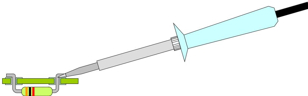
This diagram shows a component mounted on a printed circuit board about to be soldered. The tip of the soldering iron is correctly placed to heat the lead and the printed circuit just prior to applying the solder.
